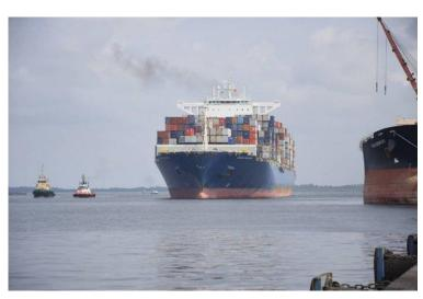
The Maerskline Stardelhorn vessel that arrived Onne with Length overall of 300 metres, width of 48 metres and capacity of 9,971(TEUs).
